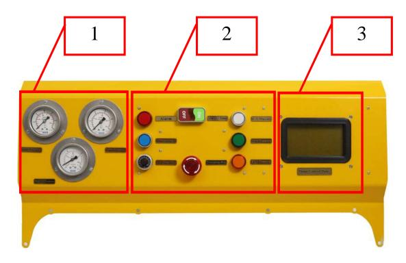
1)Manometers: In this section, there are 2 manometers to show the Pressure of the pump in 2 stages. The first one shows low pressure, the second shows Low pressure.
